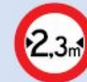
C18 No access for vehicles with a width, including the load, greater than indicated
